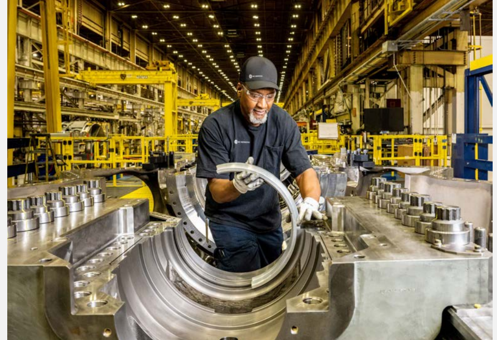
Assembler with a 7HA.03 gas turbine in Greenville, SC
